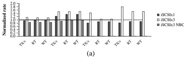
**Figure 7.** Postmark results normalized to the direct configuration. Each graph represents one input size. Each group of bars refers to one application metric: Transactions/s, Read Throughput, and Write Throughput. Each bar refers to one system configuration: direct, iSCSIx1, iSCSIx3 and iSCSIx3 without buffer cache (left to right).
